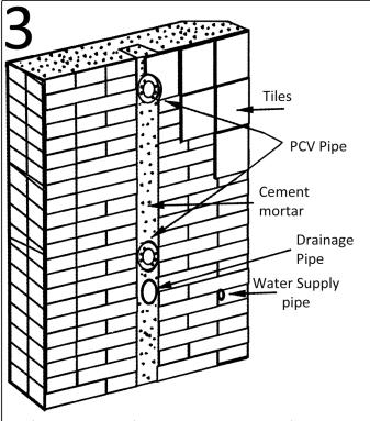
Fix the PVC pipe with cement mortar, once this is complete, you can start your tiles.
