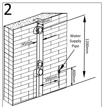
Slot the wall according to the figure, then place the PVC elbow into the slot.
