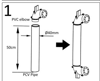
Prepare a white PVC drain pipe in advance accoring to the size above. Put the PVC elbow into the PVC pipe.
