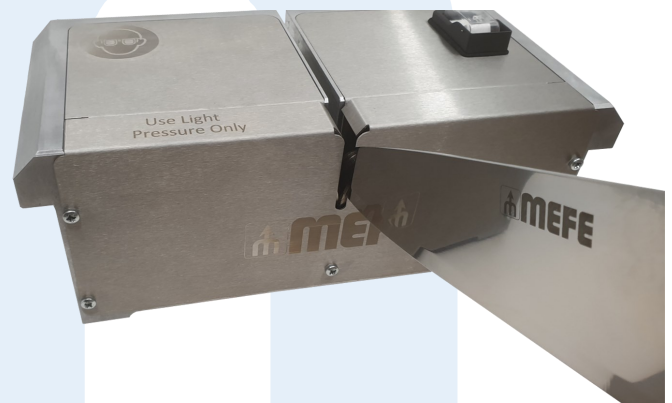
Figure 4—Showing end of grinding operation, lifting knife away from the grinding wheels
