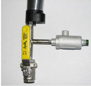
Figure 4: Vacuum Transducer installation detail
