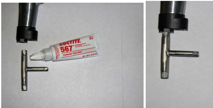
Figure 2: T-Pipe installation detail
