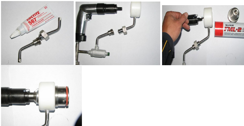
Figure 5: S-Pipe installation detail & White Air Collar
