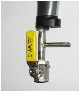
Figure 3: Ball Valve installation detail
