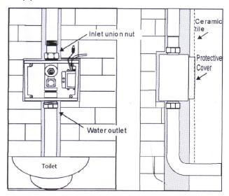
4. Open the battery holder and insert 4 x AA alkaline batteries. Connect sensor panel, power cables and solenoid valve. Put the power adapter and battery holder back into the mortar. When the power is turned on, the LED light will flash once.
