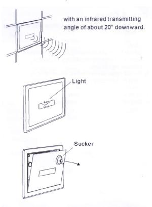
Note: The sensing distance is set 70cm away from the sensing window, along the direction of the transmitting angle. Transmitting angle of 20° downwards.
