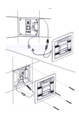
Please check interface for leaks during water pressure test. Grout the gap between control box and the wall and stick tiles down. Once grout is dry, remove and dispose of protective cover.
