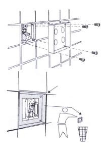
5. Screw the fixed panel with 4 long screws and cover the panel.
