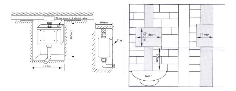
2. Please clean impurities and silt from pipeline. Screw down the water inlet nut and connect to pipeline.
