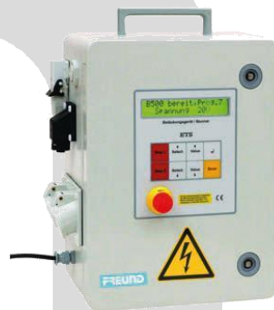
CAT 44 E514 High volume constant amperage stunner or killing device for constant operation (high frequency). Individual programming allows usage as a E-stunner or a killing device for killing of pork, beef and sheep in the case of epidemics or casualties. 2.5amp; 18kg.
