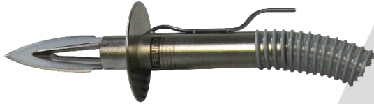
Sticking Knife With Anti Coagulation Tube
