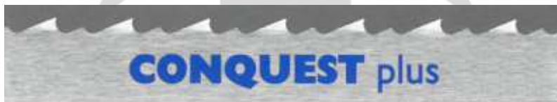
Conquest plus – produces a clean and even cut through improved removal of cutting waste , Developed for abattoir Splitting Bandsaws for speed and longevity. 2.5 teeth per inch
