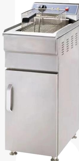
Capacity: 6 + 6L Voltage: 220-240V Power: 2.5 + 2.5kW Weight: 9kg 550 x 460 x 300mm 2 Basket Countertop Fryer CAT 6622B
