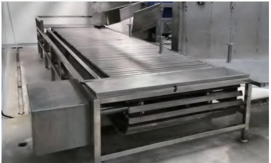
CAT 55-BCS5 Sticking, Bleeding Conveyor 5M Long
