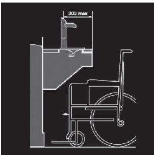
Font installation to accommodate disabled access.
